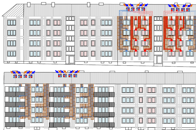
Fig. 4 Positioning of ventilation ducts for Site 2
