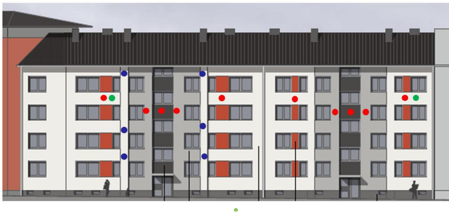
Fig. 6 – Pt 100 sensor positioning front of the building
