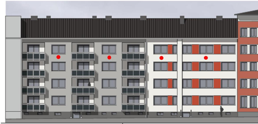
Fig. 7 – Pt 100 sensor positioning back side of the building
